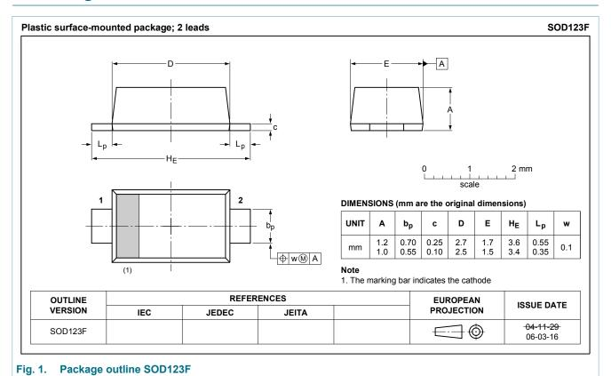
plastic, surface-mounted package; 2 leads; 2.6 mm x 1.6 mm x 1.1 mm body
