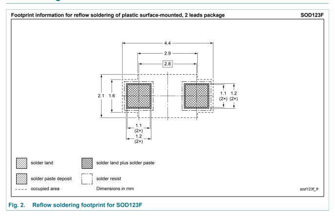
plastic, surface-mounted package; 2 leads; 2.6 mm x 1.6 mm x 1.1 mm body
